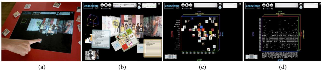
**Figure 1:** The *collecTable* running on the *iTable* (a), with several fiducials over it. The digital projections of the fiducials floating over the interface (b), each fiducial storing different music collections. The *M-Cube* interface for music data showing albums (c) and tracks (d).
